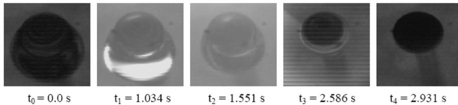
Fig. 3 Biodiesel Droplet Burning Sequence
