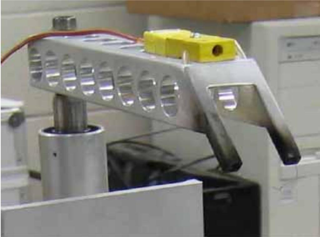
Fig. 2. Thermocouple Arrangement for Droplet
