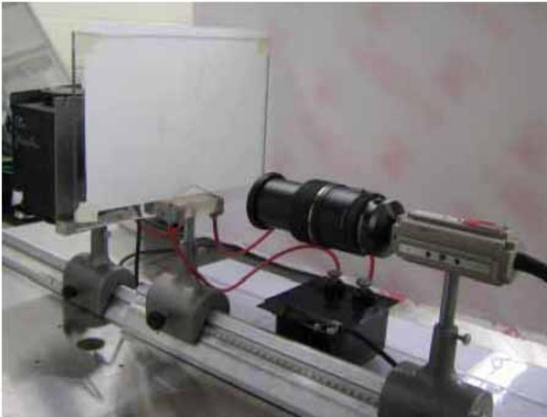
*Fig. 1. Optical Apparatus for Determining Droplet Diameter*
