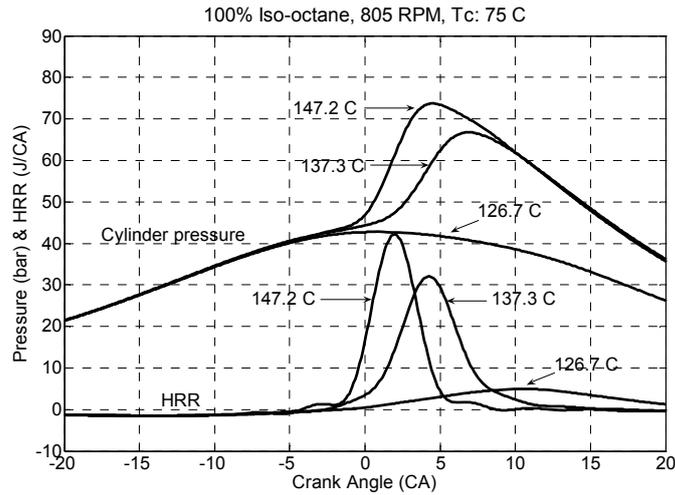
Fig. 4. Cylinder pressure and rate of heat release at different intake charge temperatures (805 RPM, 100% Iso-octane)
